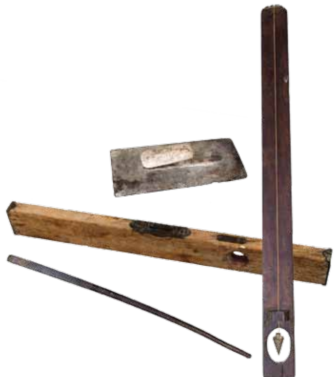
A Capitol construction worker used these tools as a stonemason, clockwise from top right, plumb bob, tamping bar, mason's level, and float.
